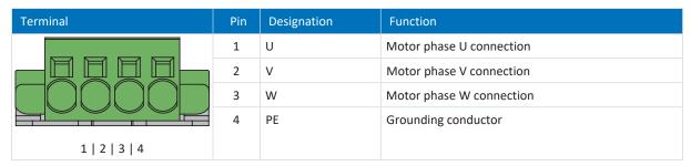
Tab. 141: X20A connection description, sizes 2 (double-axis controllers) and 3
